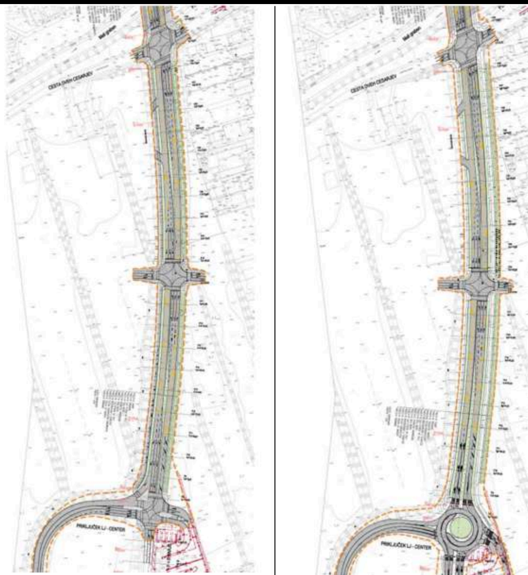
Conceptual design – reconstruction of Barjanska cesta from Zihierlova ulica to the Crossroads with highway connection center and P+R (park and ride) Barje (LUZ d.d., project no. 8359 Left: variant 1, right: variant 2)
